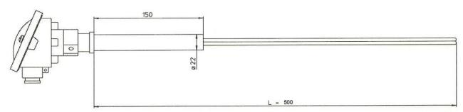
Based on the specified max leaking rate of 1,0E-06 mbar-liter/s this thermoelement has passed the test and is released for the use in vacuum furnaces.
